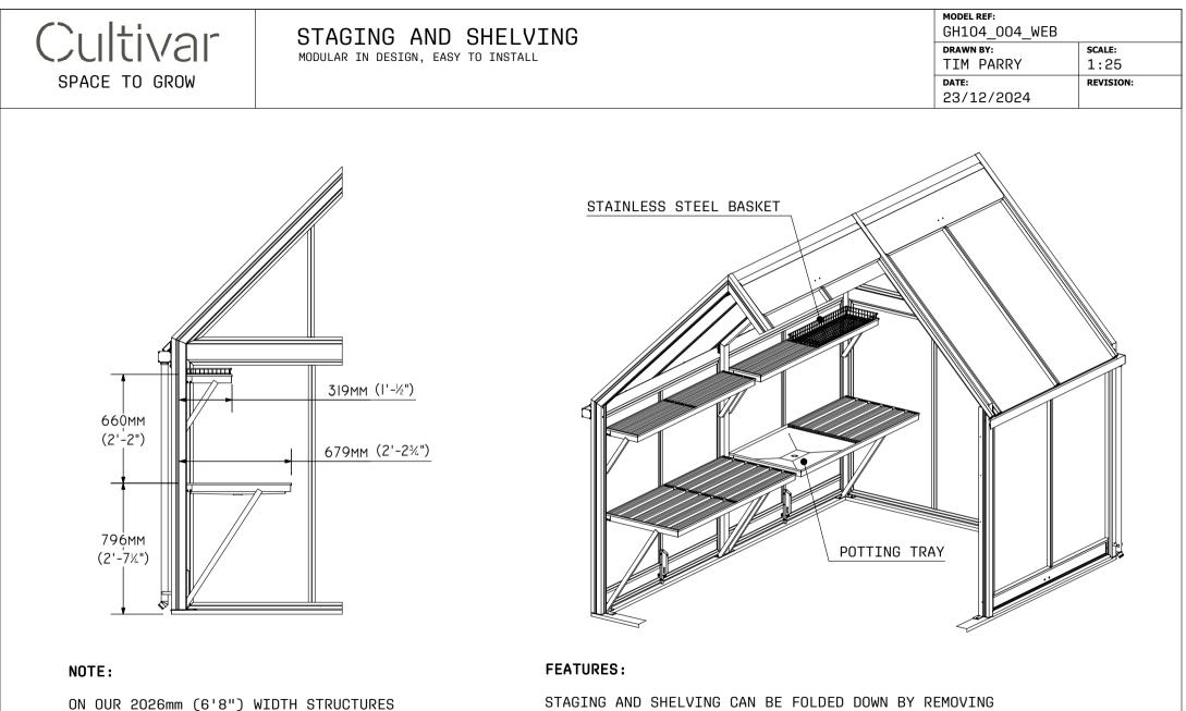
ON OUR 2026mm (6'8") WIDTH STRUCTURES THE STAGING WIDTH IS 570mm (1'11") STAGING AND SHELVING CAN BE FOLDED DOWN BY REMOVING STAYS PROVIDING EXTRA FLOOR SPACE WHEN NEEDED.
